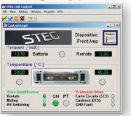
With the aid of a simple and intuitive graphic interface, MY STEG MANAGER displays the status of the amplifier in real time on the monitor screen, relaying essential operational parameters such as: power supply and remote/on voltage, running temperatures (right and left side of the heat sink), status of the cooling fans and, most of all, a detailed roundup of the protections system. By
